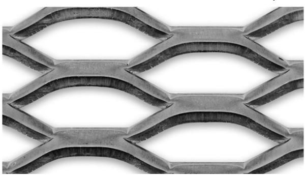
LW Pitch:121.92mmStrand Width:9.53mmSW Pitch:35.85mmThickness:6.00mmWeight:24.98 kg / m2Open Area:47%
